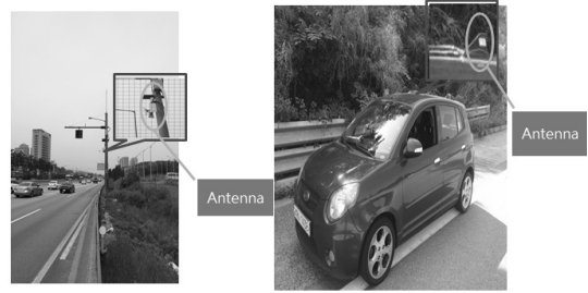
<Fig. 1> RSS communication module and OBE communication module antennas
