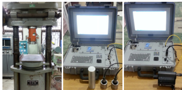
(a) Compressive (b) UPV (c) Impact Echo
