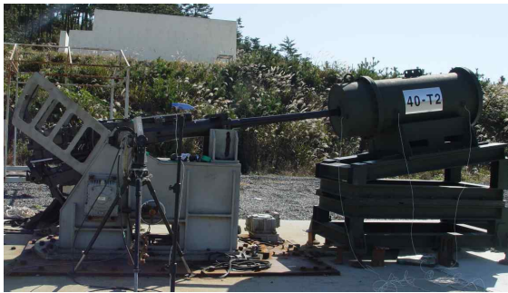
Fig. 9 The installation of muffer to 40 mm medium caliber gun during the fire
