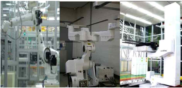
Fig. 1 A kind of the substrate handling robot with forks
