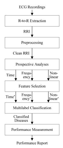
Fig. 1. Proposed method for automated diagnosis of various diseases.
