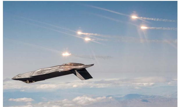
Fig. 8 F-35 Flare Release During Flight Test
