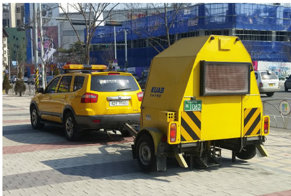
Fig. 1 Falling Weight Deflectometer (FWD)
