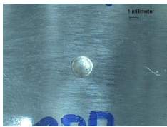
(b) Particle diameter: 2 mm, Impact velocity: 877 m/s
