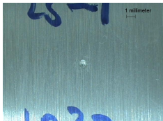
(a) Particle diameter: 1mm, Impact velocity: 1032m/s
