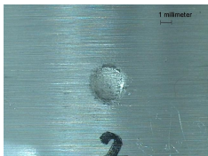
(c) Particle diameter: 3mm, Impact velocity: 1032m/s
