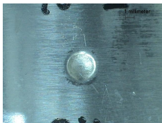
(c) Particle diameter: 3 mm, Impact velocity: 811 m/s
