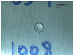
(b) Particle diameter: 2mm, Impact velocity: 1008m/s
