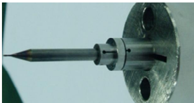
Fig. 1 Shape of tool holder based on SMA
