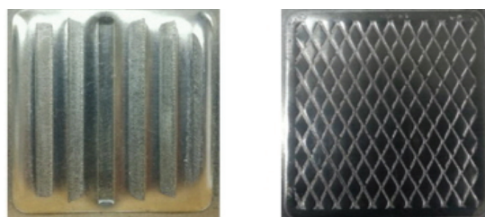
Fig. 7 Emboss patterns formed using an electromagnetic force 71
