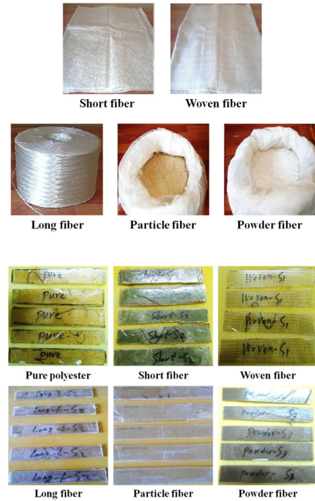
Fig. 7. Overview pictures for types of composites glass fiber and composite materials[22].
