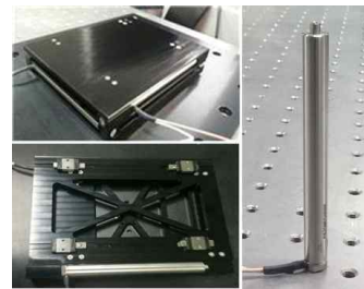
Fig. 1 PZT focal plane compensation device(left) and PZT actuator(right)
