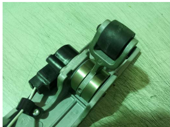
Fig. 6. Accelerator return bearings and roller
