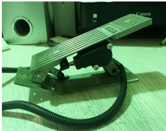
Fig. 1. APP (Accelerator Pedal with APS)
