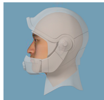
Fig. 8 Modeling of a fire helmet
