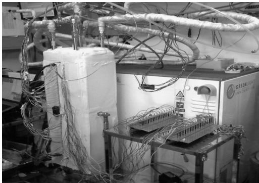
Fig. 6 5 kW HT-PEMFC stack operation for long term durability test with cell voltage control device
