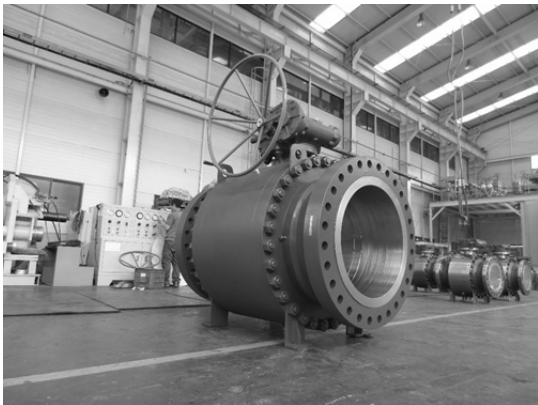
Fig. 2 Prototype of a 30 inch ball valve
