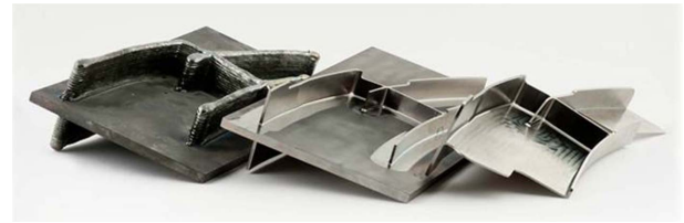
Fig. 1. Example of post-processing of directed energy deposition AM product.
