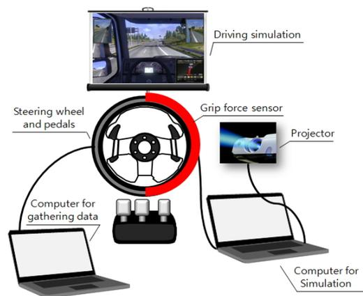
Fig. 2. Simulated driving task diagram
