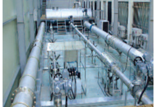
Fig. 3 Measurement system for flow coefficient
