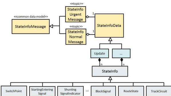
Fig. 10. Mapping Related 'Message Type' model of KRS SG 0062 to 'StateInfoMessage' model
