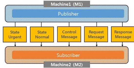
Fig. 15. Experiment Design of Data Transmission of Conventional Railway Signal Data
