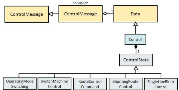
Fig. 11. Mapping Related 'Message Type' model of KRS SG 0062 'ControlMessage' model
