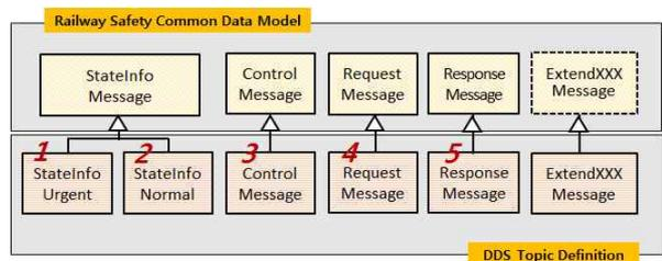
Fig. 4. Mapping Railway Safety Common Data Model to DDS Topic Definition
