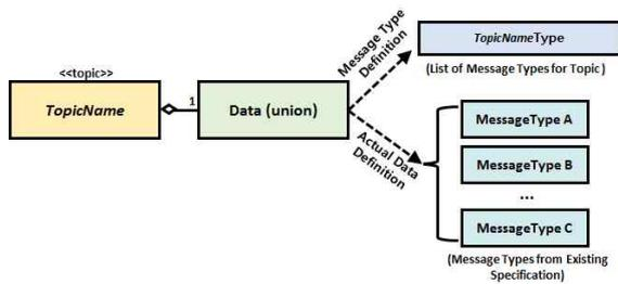
Fig. 5. Data Transformation Process #1 - Including Multiple Message Types
