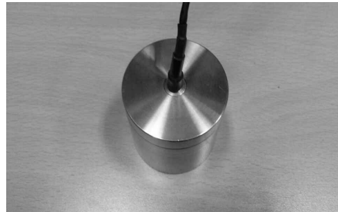
Fig. 3. Ultrasonic Sensor with a Waterproof Case
