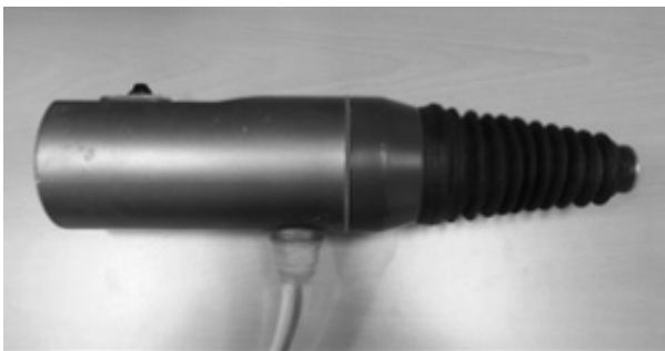
Fig. 2. Schmidt Hammer with a Waterproof Case
