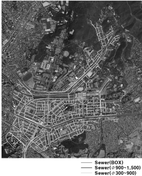
Fig. 3. Storm Sewer of Shinchon
