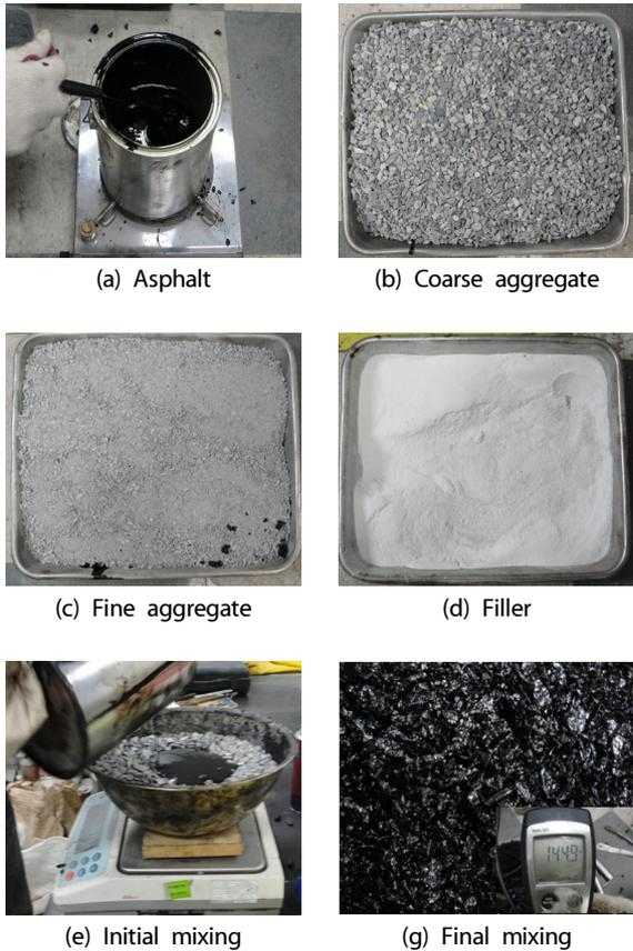
Fig. 3. Mixing process of asphalt
