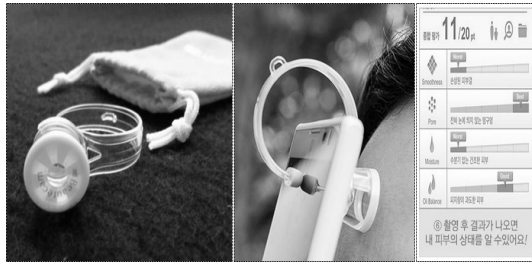
Fig. 2. The picture of BauteCam device and the diagnosis result using the application.
