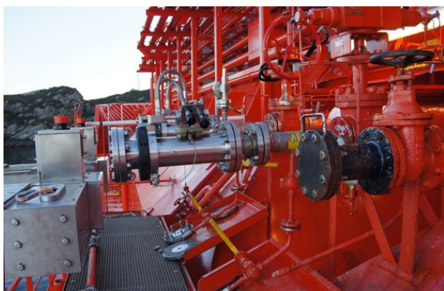
Fig. 4. Emergency release system (ABS, 2015).
