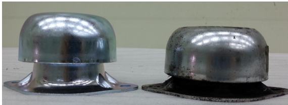
Fig. 1. Deformation of APU metal mount
