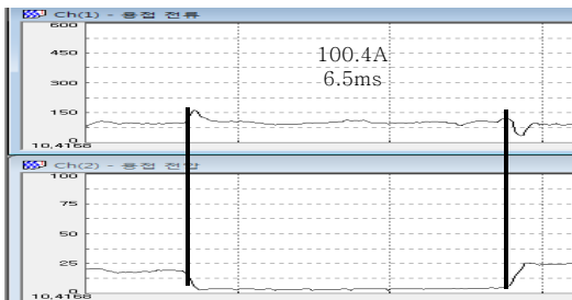
Fig. 6 Waveform analysis of domestic welding power source A at 90A
