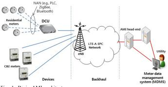
Fig. 1. Basic AMI architecture
