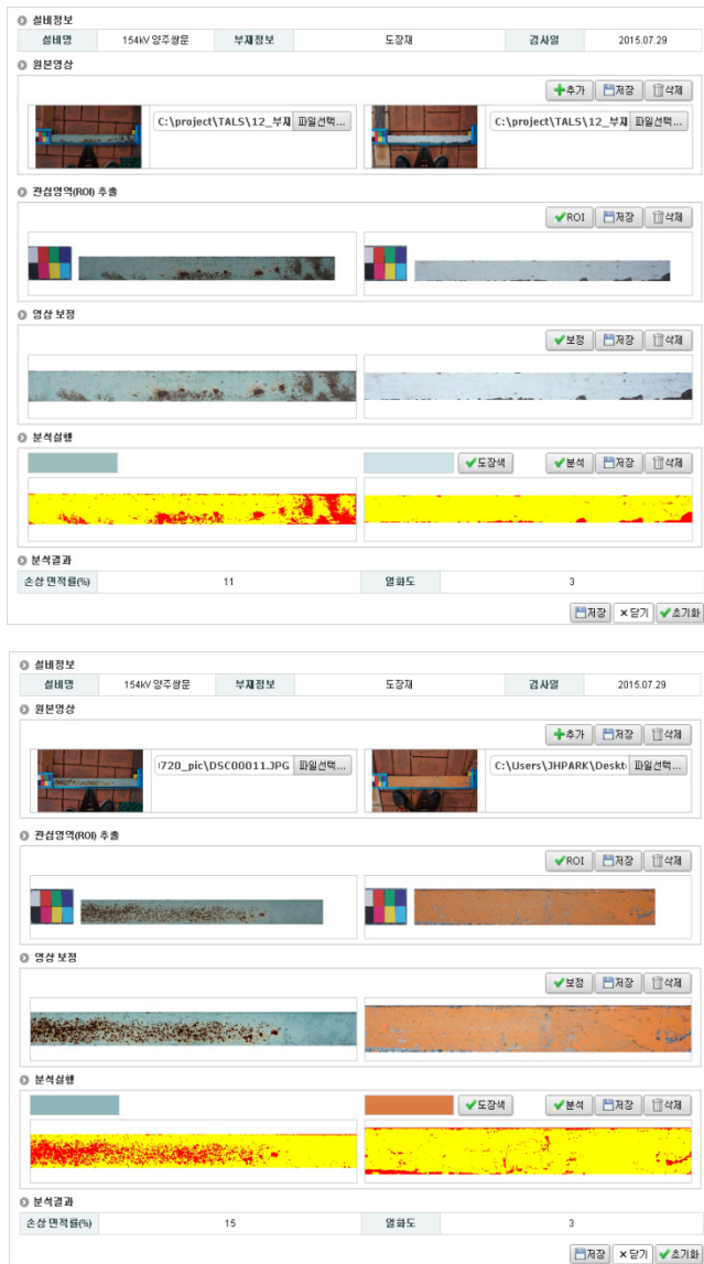
Fig. 8. Analysis result of corrosion deterioration for transmission tower painted member.
