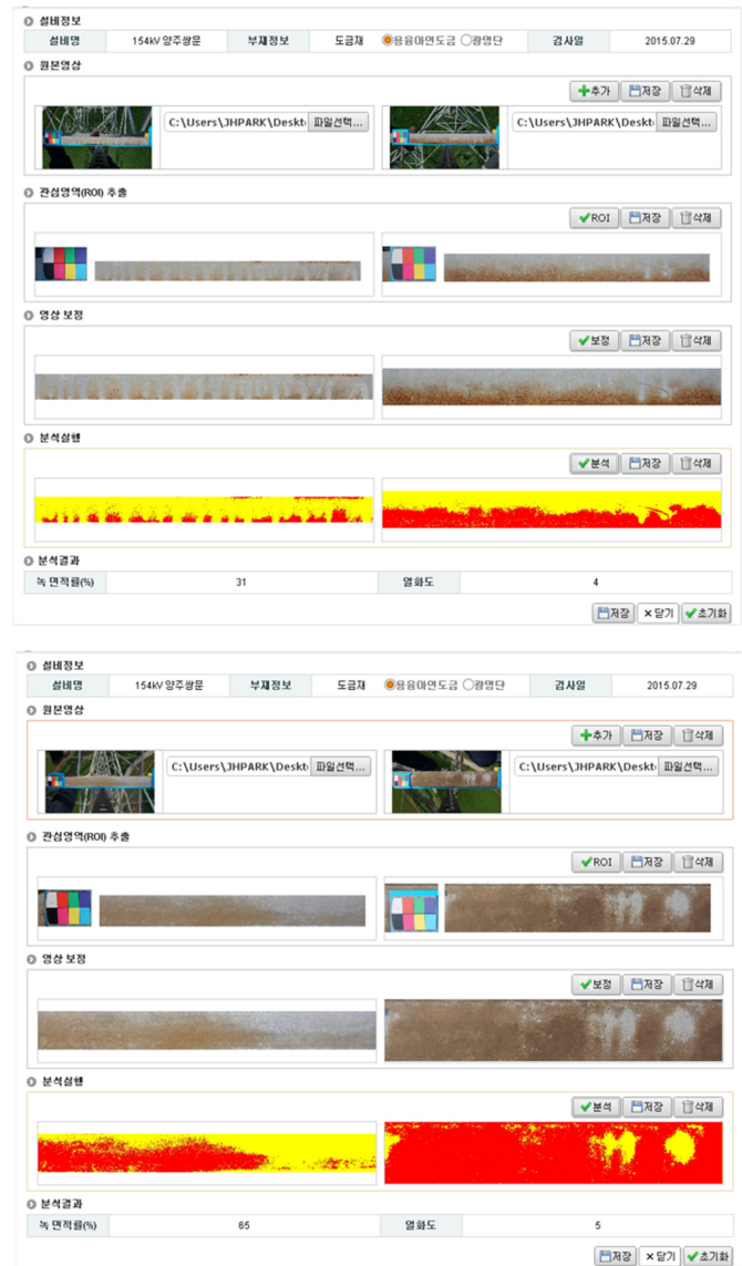
Fig. 7. Analysis result of corrosion deterioration for transmission tower hot dip galvanizing member.
