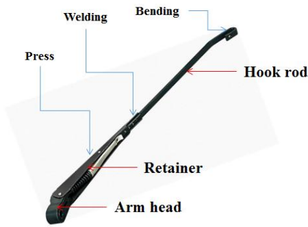
Fig. 1 Structure of window wiper
