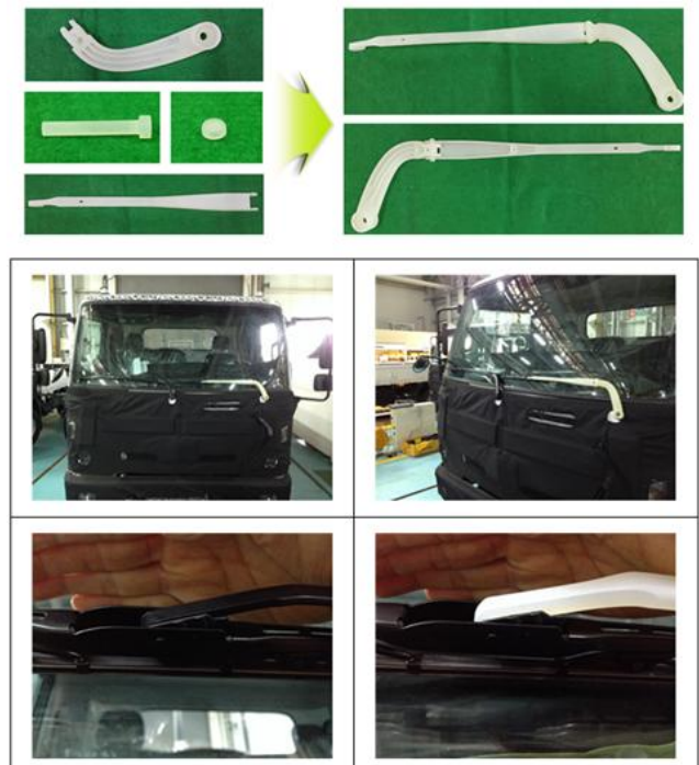
Fig. 12 Rapid prototype manufacturing and interference test for heavy truck
