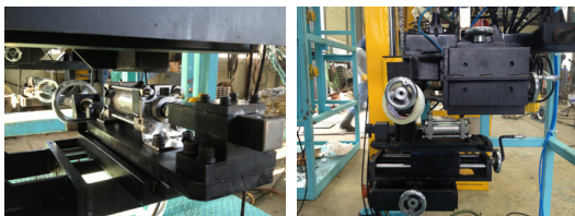
Fig. 13. Welding carriage equipment
