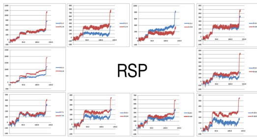
Fig. 17. Shrinkage length change of concrete specimen and with using shrinkage reducing agent
