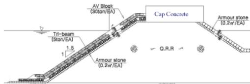
Fig. 7. Drawing of a breakwater with AV block
