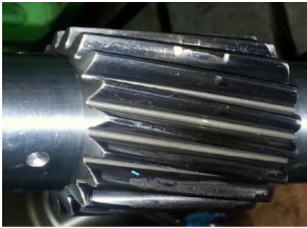
**Fig. 10** Damaged teeth of pinion
