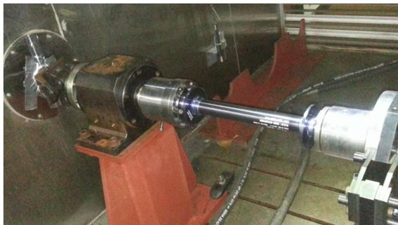
Fig. 14 Static torsional test rig
