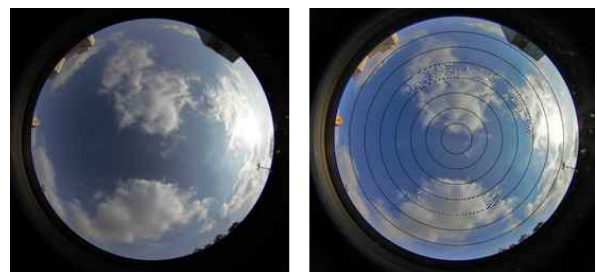
Fig. 7. Original sky image and the corrected image (F11)
