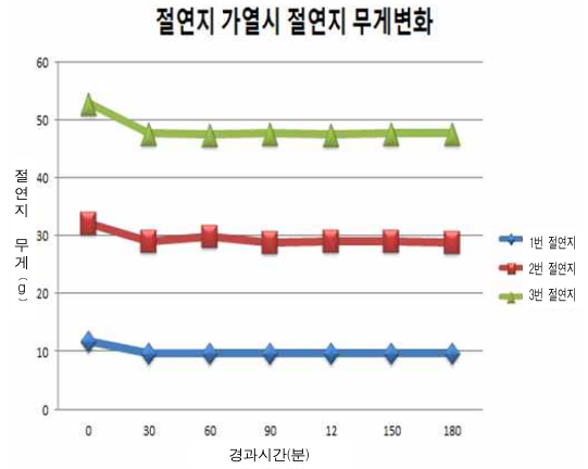
Fig. 1. Insulation paper weights according heating time
