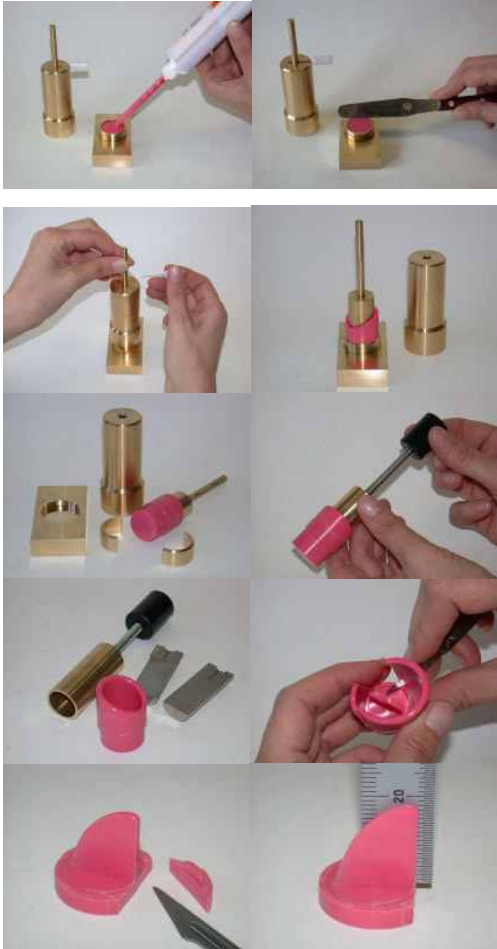
Fig.2. Shark fin test device and procedure for measurement[4]
