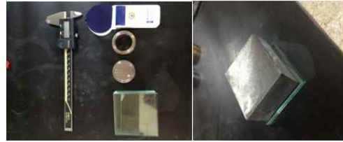
Fig.1. Apparatus for consistency and elongation measurement
