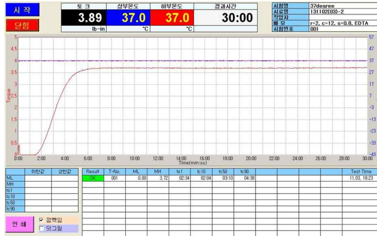
Fig 1. Typical graph of Rheometer (Model DMR 200) for setting time measurement
