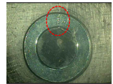
Fig. 10 Picture of heat treated process & head bolt scale for SCM435
