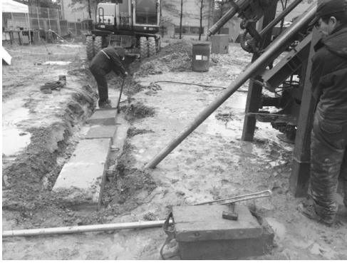
Fig. 6. Field drilling tests for reinforced concrete specimens
