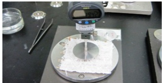
Fig. 4. Measuring thickness of the vegetation mats
