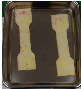
Fig. 6. Tensile specimens of PLA plastic
