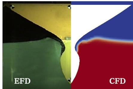
Fig. 18 Bow model free surface t = 0.25 s
