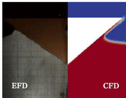
Fig. 13 Stern model free surface  $t = 0.355$  s
