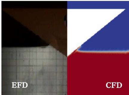
Fig. 11 Stern model free surface  $t = 0.325$  s
