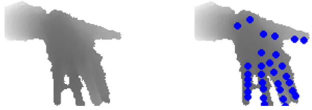
Fig. 2. Input (raw) and output (estimated) hand poses.
