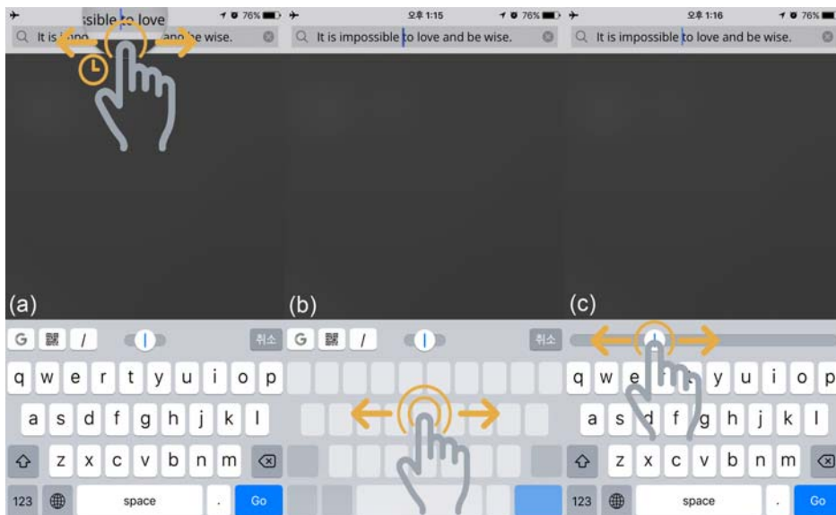
Figure 2. Three types of cursor control in opera mini browser(each follows (a) Default, (b) 3D Touch, (c) Slide)
