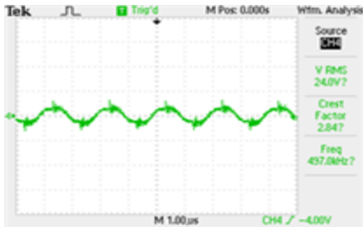
Fig. 7. Result of the waveform for the intensity (1–10) of the output voltage of Monopolar Mode 3 (RET, 500 kHz).
