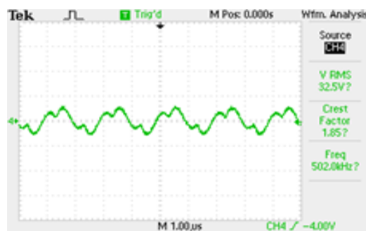
Fig. 6. Result of the waveform in intensity (1–10) of the output voltage of Monopolar Mode 2 (CET, 500 kHz).
