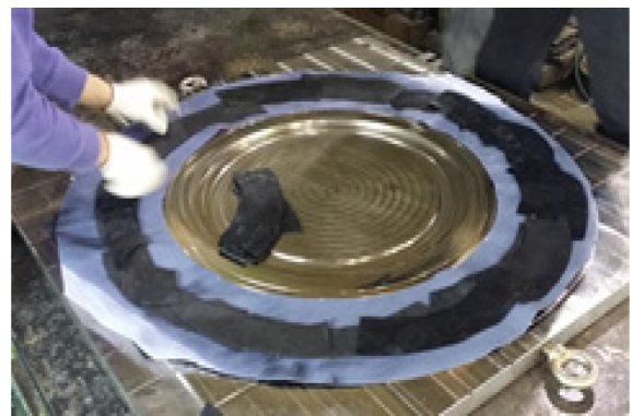
(b) Manufacturing process of air tube
