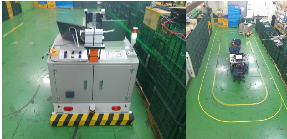
Figure 1. Experimental setup for navigation of the moving target
