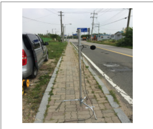
<Fig. 5> Implemented microphones for measuring noise
