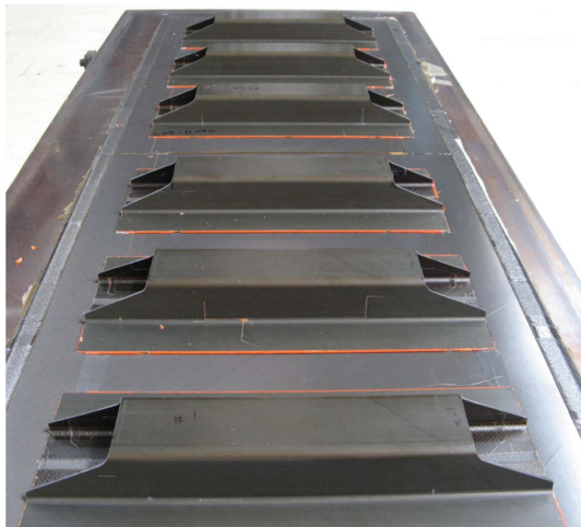
Fig. 5. Co-bonded Panel specimen with caul plate
