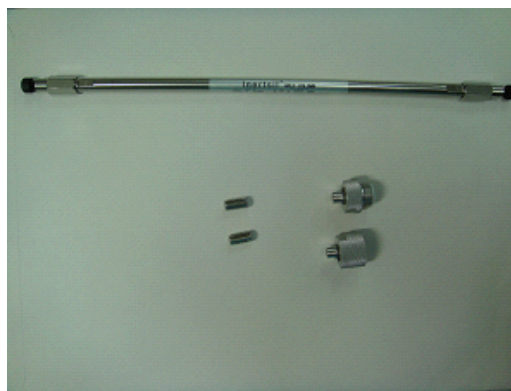
Fig. 1. HPLC main column (upper), guard column (below left), and guard column holder (below right).
